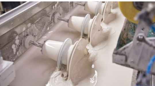
Nowadays, state-of-the-art machines dip the plates and cups into the glaze with the utmost precision.
