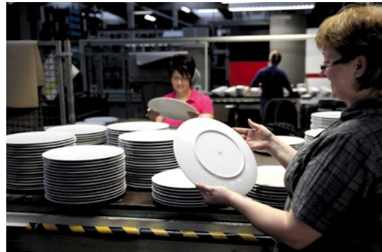
Careful inspection: the finished white ware is sorted in accordance with rigorous quality standards.
