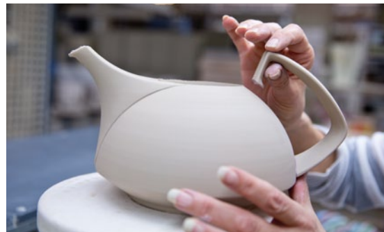
Many items must still be attached by hand today in spite of state-of-the-art production methods.
