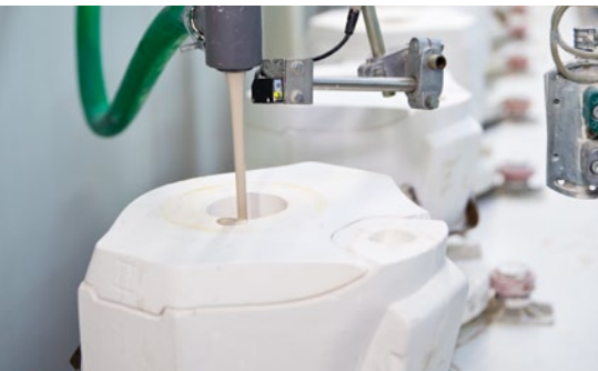
The plaster mould is filled with the liquefied porcelain paste, known as the slip.
